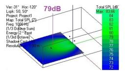
Figure VII. Placing two traditional loudspeakers we get 79dBspl.
